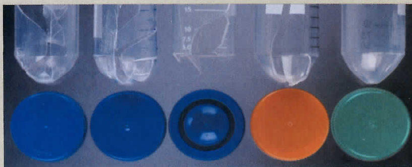
Comparison photo of 50mL tube cones shows thicker cones of SuperClear tubes (far right, Teal) withstand breakage better than popular brands. Actual test with market samples. Tubes filled with 45mL distilled water. Spun unsupported for 15 minutes @ 20,000 RCF.
